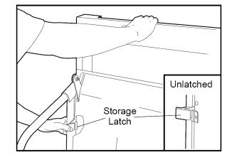
2. Hold the treadmill firmly with both hands, and lower the treadmill to the floor. Do not drop the treadmill frame to the floor. To decrease the possibility of injury, bend your legs and keep your back straight.
